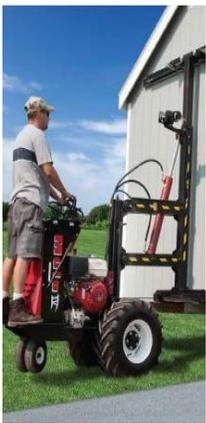
The Mule operator lifts one end of the shed using the simple controls so the dolly wheels can be positioned.
